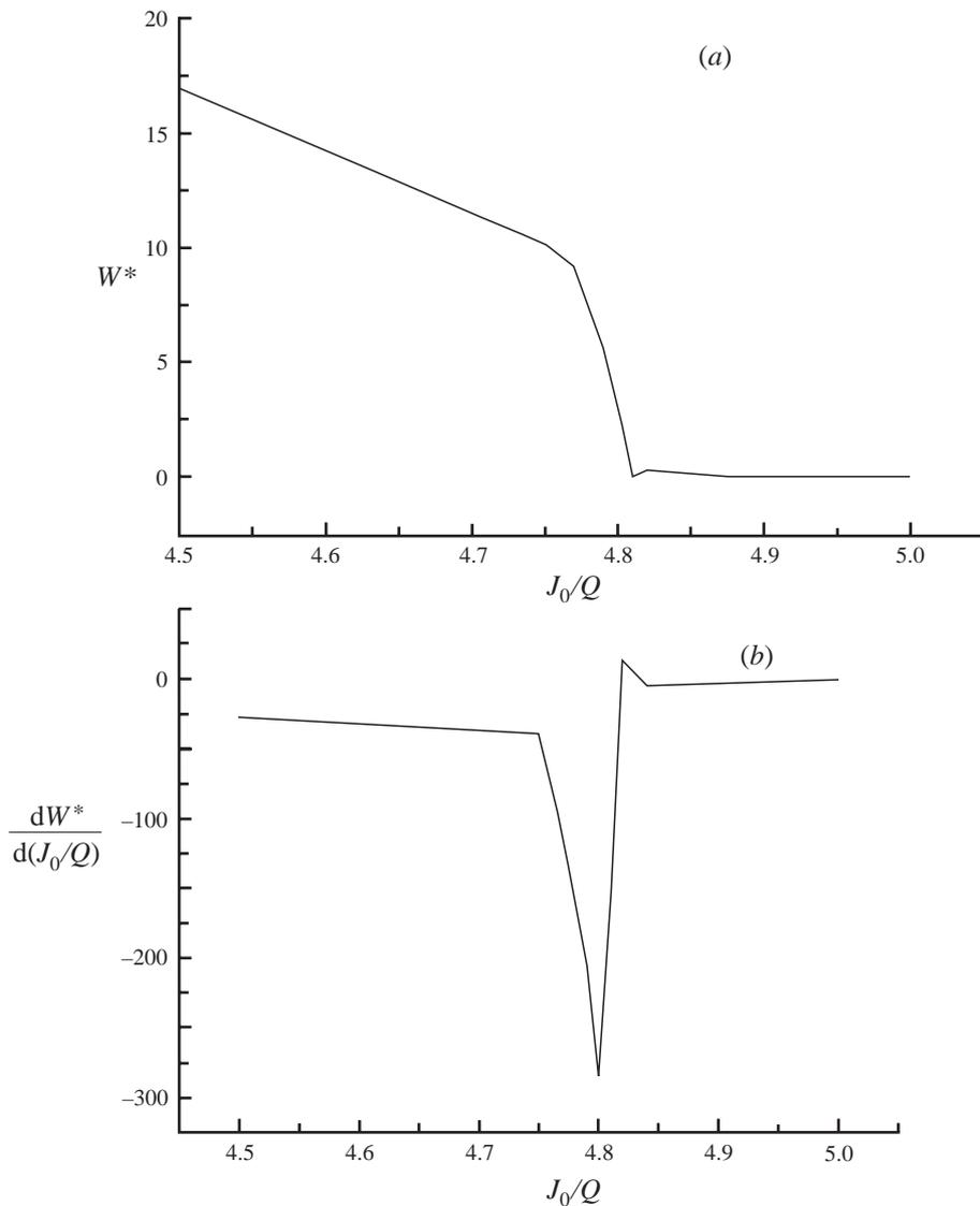
FIGURE 7. (a) Root-mean-square average of the dimensionless vertical water velocity and (b) its derivative with respect to  $J_0/Q$  both as a function of  $J_0/Q$ .
