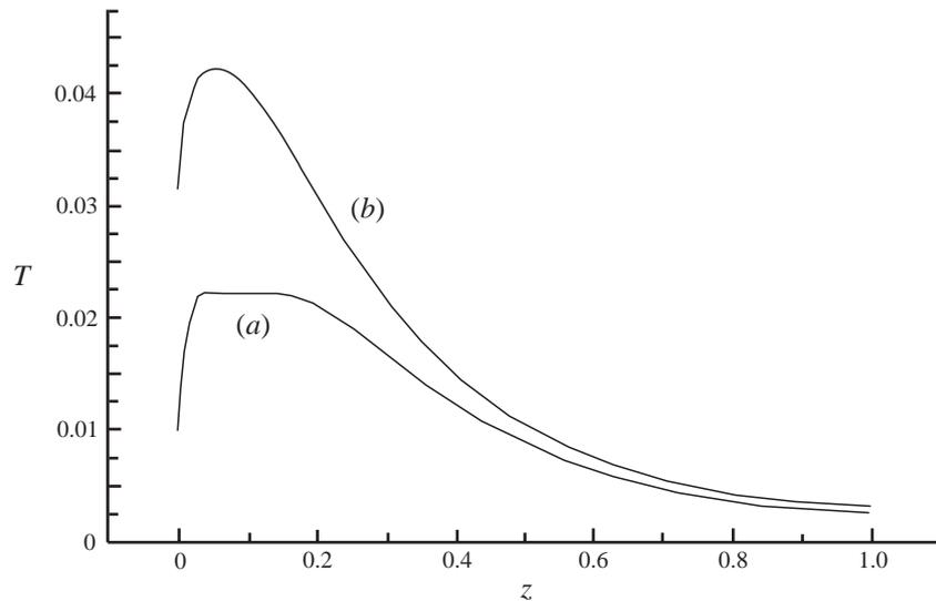
FIGURE 6. Vertical profiles of the horizontal-average dimensionless water temperature at  $R = 5 \times 10^8$ ,  $N = 102$ ,  $N_0 = 55$ ,  $\beta_0 = 1.1 \times 10^6$ : (a)  $J_0/Q = 4$ ,  $a = 36.7$ ; (b)  $J_0/Q = 4.75$ ,  $a = 34.8$ .
