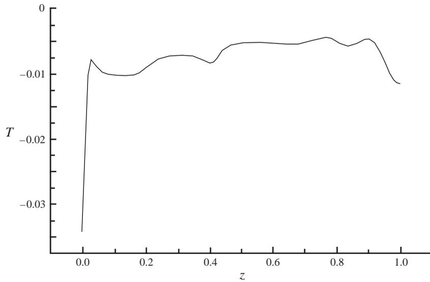
FIGURE 3. Vertical profile of the horizontal-average dimensionless water temperature at  $J_0/Q = 1.5$ ,  $R = 5 \times 10^8$ ,  $N = 102$ ,  $N_0 = 55$ ,  $\beta_0 = 1.1 \times 10^6$ ,  $a = 42.5$ .
