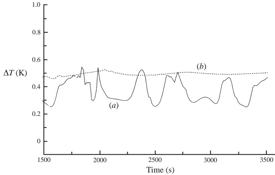
FIGURE 2. Horizontal-average dimensional temperature drop across the cool skin at  $Q = 100 \text{ W m}^{-2}$ ,  $R = 5 \times 10^8$ ,  $N = 102$ ,  $N_0 = 55$ ,  $\beta_0 = 1.1 \times 10^6$ , where (a)  $J_0/Q = 1.5$ ,  $a = 42.5$ ; (b)  $J_0/Q = 1.9$ ,  $a = 41.5$ .
