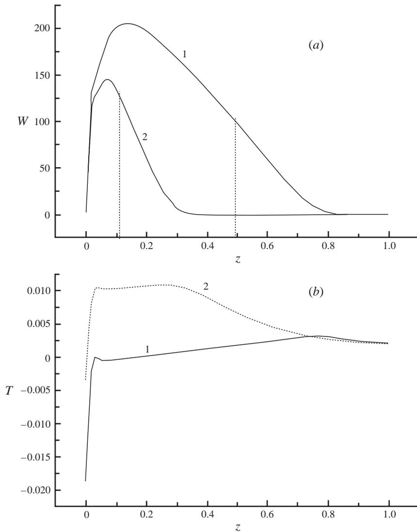
FIGURE 5. Vertical profiles of (a) the horizontal root-mean-square average of dimensionless water velocity and (b) the horizontal-average dimensionless water temperature at  $R = 5 \times 10^8$ ,  $N = 102$ ,  $N_0 = 55$ ,  $\beta_0 = 1.1 \times 10^6$ : (1)  $J_0/Q = 2.6$ ,  $a = 40.4$ ; (2)  $J_0/Q = 3.5$ ,  $a = 37.8$ . In each case, dotted lines bound the sublayers of thermal compensation.
